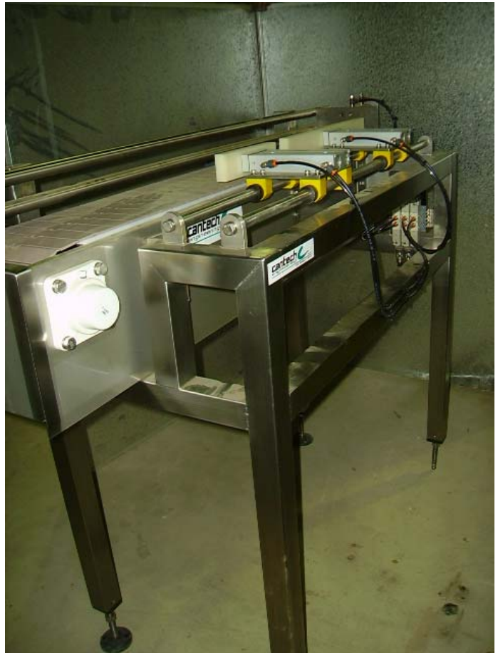
Manifold mounted valves reduce assembly time
